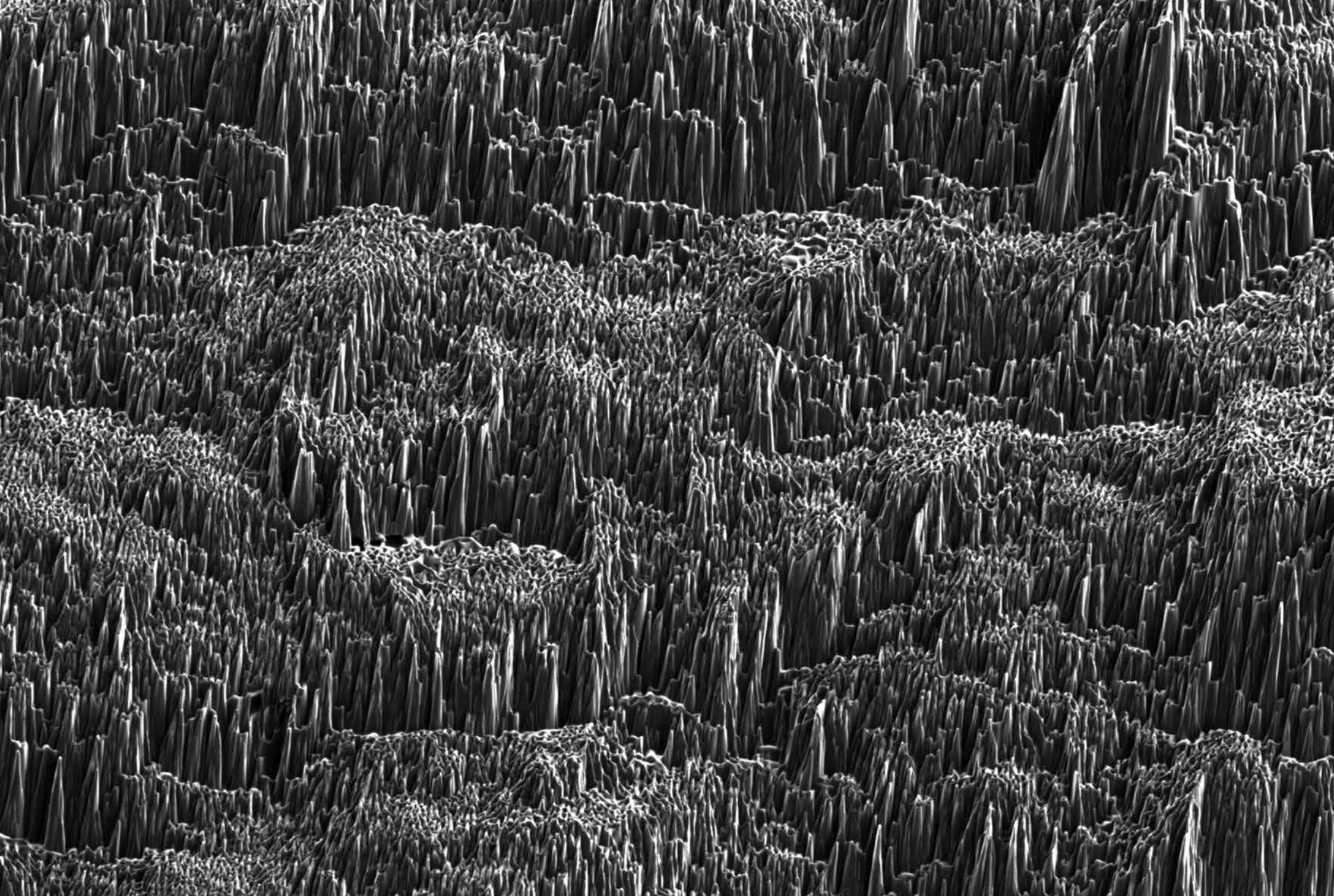
Graphene oxide fiber after Ga + ions milling, FIB image (KZ, 2 500x) 65
